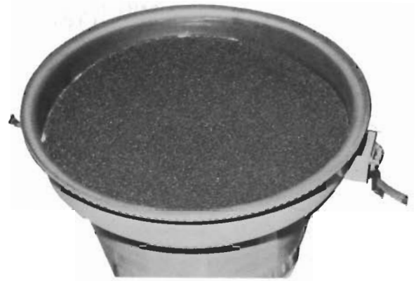
Fig. 12-C The hopper filter has two distinct sides, one made of a sateen cloth, one of a urethane foam. The urethane side fits against the expanded metal support in the hopper cover. Properly installed, the filter's urethane foam side is up.
