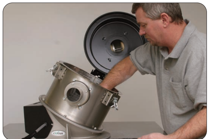
Angled receivers make it easier for operators to reach inside for cleaning or maintenance.
