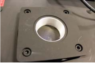
Filter Screen Within the Vacuum Inlet to the Pump
