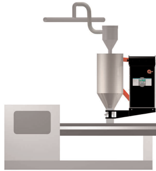
Dryer and hopper on the processing machine throat using the optional support frame.
