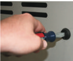
Dryer Door Locking Bolts (2) (W1600-5000)
