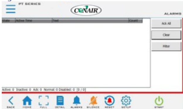
Figure 8 – HMI Alarm Handler
