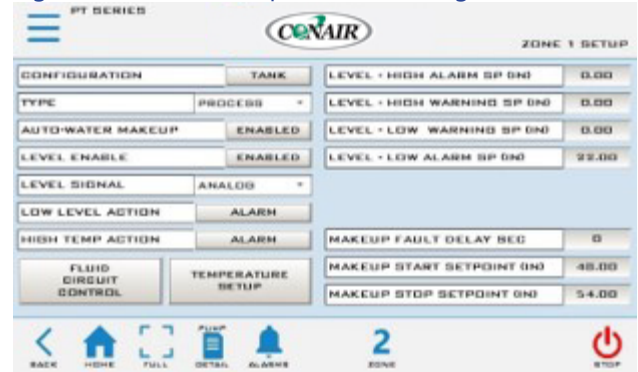
Figure 10 – Zone Setup Screen (Analog Level Sensor)
