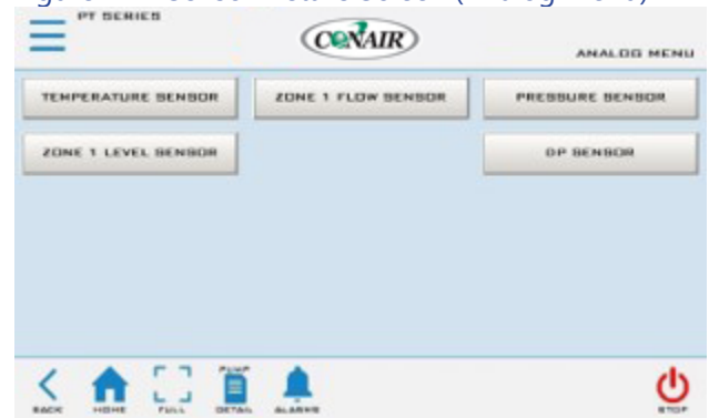
Figure 21 – Sensor Details Screen (Analog Menu)
