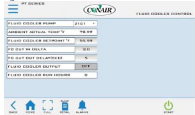
Figure 44 – Fluid Cooler Screen
