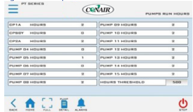
Figure 34 – Pumps Run Hours Screen
