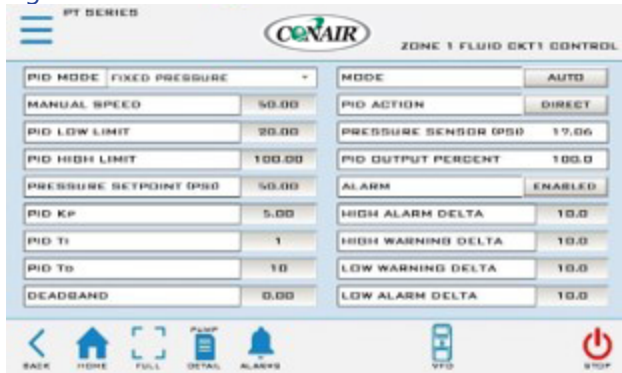
Figure 12 – Zone X Fluid Circuit X Control Screen
