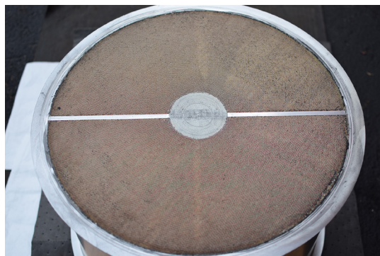
Example of a Desiccant Rotor with More Than 15% Blockage
