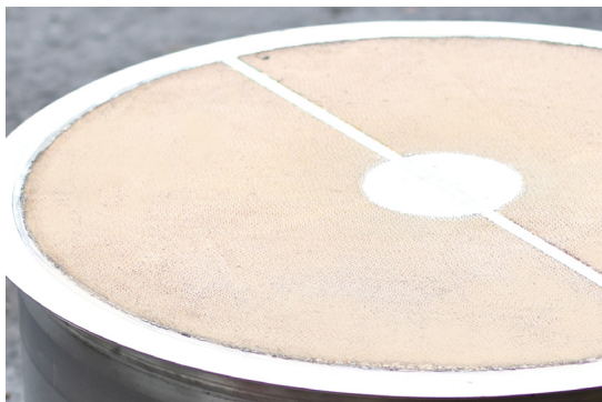
Example of a Clean Desiccant Rotor
