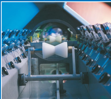
"V" Rollers accommodates multiple pipe sizes
