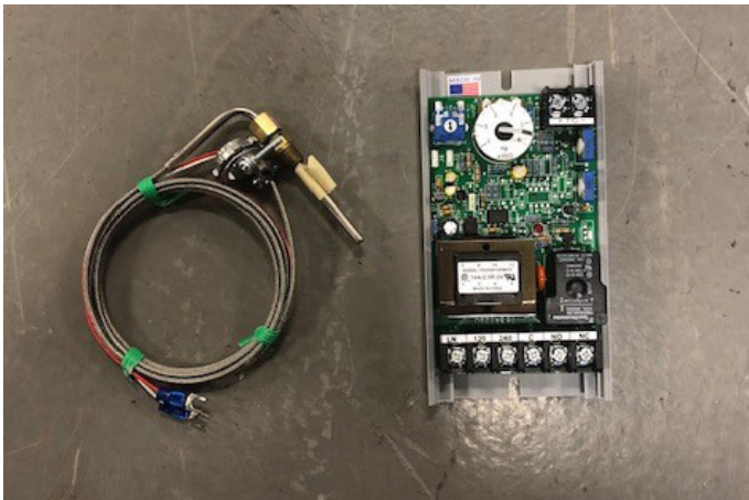
Type J Thermocouple on Left; Cut Out Switch on Right.
