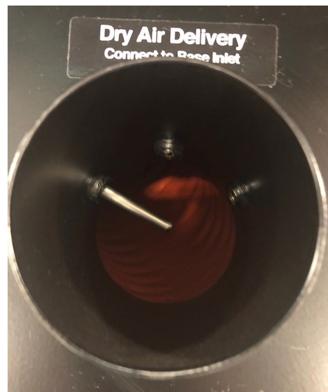
Proper Location of RTD Tip
