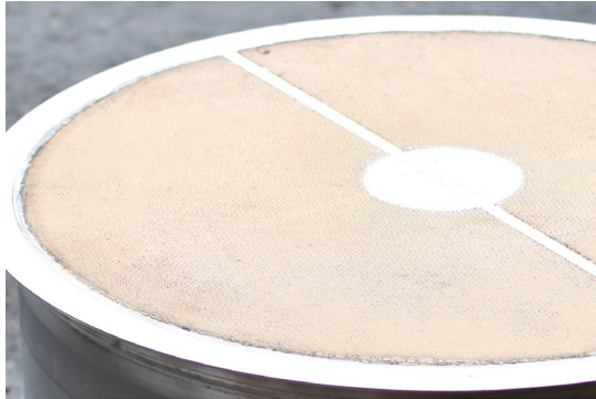
Example of a Clean Desiccant Rotor
