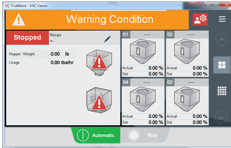
Figure 42: Alarm General Warning Alarm
