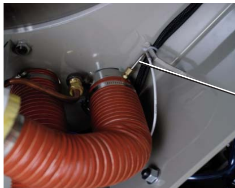
Typical location of the Process RTD at the hopper inlet.
