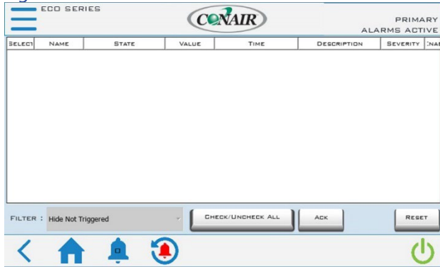
Figure 11 – HMI Alarm Handler
