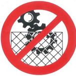
No Removal of Safety Devices and Safety Guards
