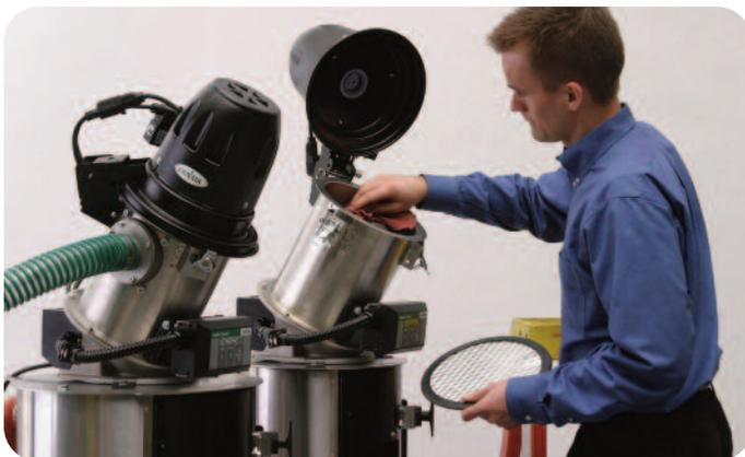
*Figure 6: Self-contained loaders use a built-in vacuum motor or venturi vacuum generator and can operate independently of a central vacuum system.*
