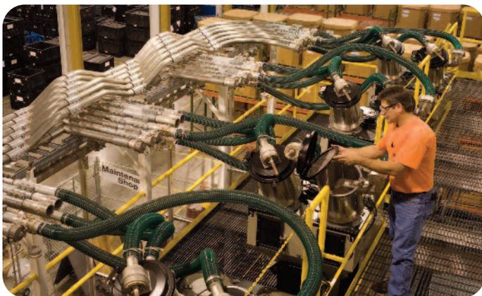
Figure 4. Vacuum material receivers, like these shown on a mezzanine above a blending station, separate plastic pellets from conveying air and deliver the resin to processing machines.
