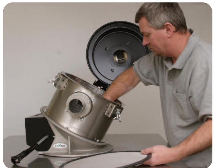
Figure 5. Conair Access receivers are angled to allow easier maintenance and cleaning.
