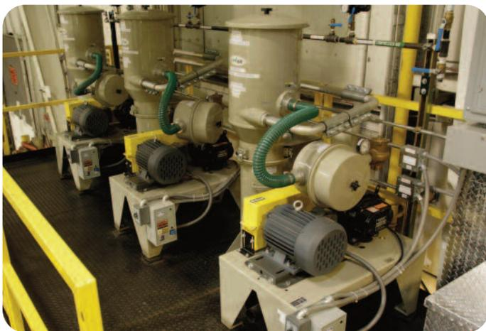
Figure 2. Providing the power behind most large central conveying systems are positive-displacement pumps like those seen here.
