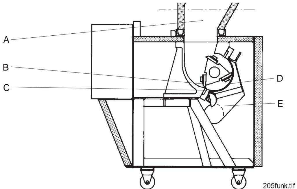
The material is fed into the hopper (A) and falls down to the rotor. The rotor's knives (B) grind the material against the fixed knives (C) in the cutter housing. Both the fixed and rotating knives can be changed or re-sharpened when necessary. The sharpening is carried out in a special fixture outside of the granulator.
