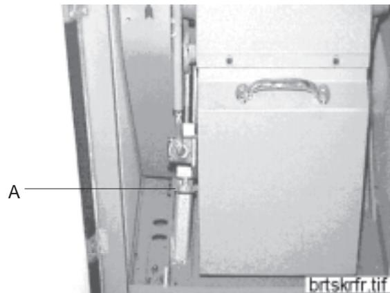
Hopper: Open the hopper as described in chapter 5.2, but close and lock the screenbox. Check the safety switch to the hopper by starting the granulator. It should not be possible to start the granulator until the hopper is lowered, the link screws are raised and the screws are tightened.
