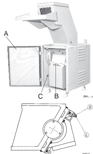
*When changing knives:* remove the screenbox completely by unscrewing from below the stop cleats under the hinge axel, after which the screenbox can be unhooked from the hinge. In this way the cutter becomes more accessible.
