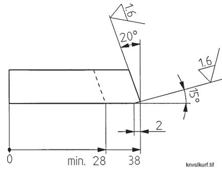
Then the knife is fastened in the 79 fixture and is sharpened to its correct cutting angle,  $15^{\circ}$ .
