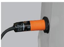
Fill sensors are provided to terminate the fill cycle and can also provide a “no material” alarm output.
