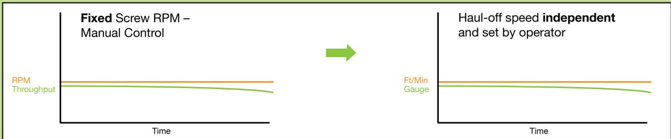
With manual line control, the extruder operates at as fixed speed and, over time, throughput drops off – as screens blind, for instance. The haul-off operates at a fixed length/time rate and, as throughput drops, gauge goes out of tolerance.
