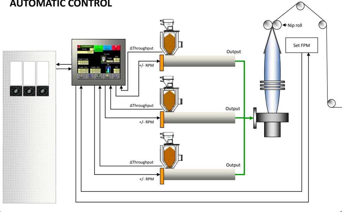
*The TrueWeigh gravimetric extrusion-line control system can synchronize material throughput, screw RPM and haul-off speed automatically to maintain maximum throughput and sheet dimensions despite changes in materials or operating conditions.*
