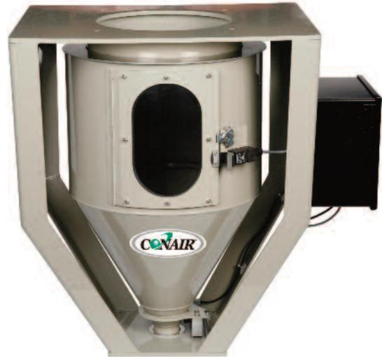
*The TrueWeigh hopper is a critical component in the Conair extrusion control system. A highly accurate load cell constantly measures the loss-in-weight of material as it flows out of the hopper and into the extruder.*
