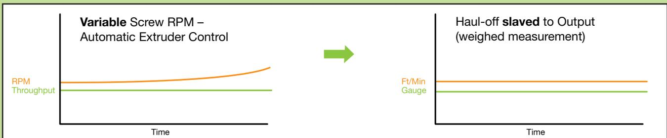
These graphs illustrate how the TrueWeigh system helps maintain throughput and gauge over time. Extruder rpm is governed according to the measured weight/hour throughput. As process conditions reduce the weight processed per rpm, the control system reacts to increase screw speed and maintain a constant weight per hour throughput. At the same time, the haul-off is slaved to the extruder throughput, changing speed as required to maintain weight/length and gauge.
