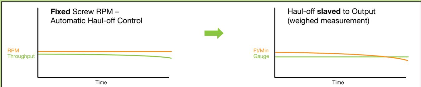
The simplest form of gravimetric control maintains a constant screw speed while monitoring throughput as it declines over time. The haul-off is then slaved to the weight/hour throughput and its speed is reduced to maintain gauge even as throughput drops off.
