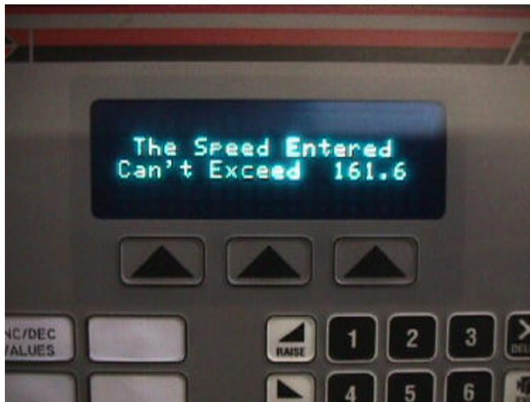
To return to the screen to enter a correct speed, push any button. Then enter a speed within the maximum limit.
