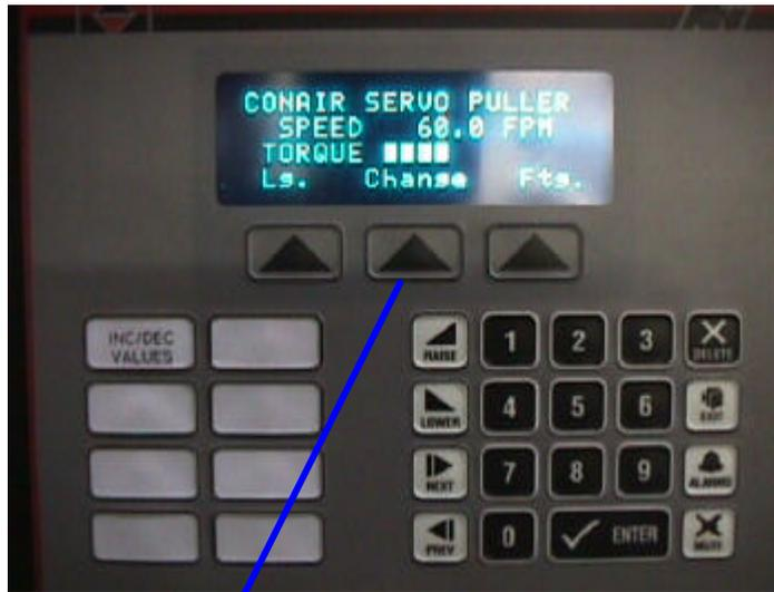
From the Sm or the Lg screen you may enter the Speed entry screen by pushing the button below the word Change
