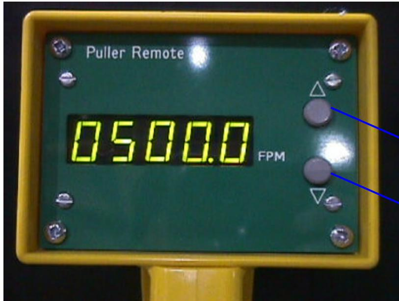
The optional remote speed control has one button with an up arrow and one button with a down arrow. Each time either of the buttons are pushed, a scroll speed change will occur at the pre-programmed value assigned to the Rm (Remote)
