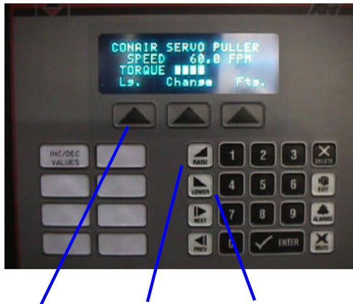
To move from the Sm to the Lg screen, simply toggle the arrow button below the Sm or Lg
