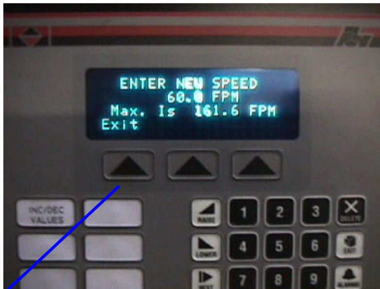
This screen allows the operator to input the actual speed desired.
