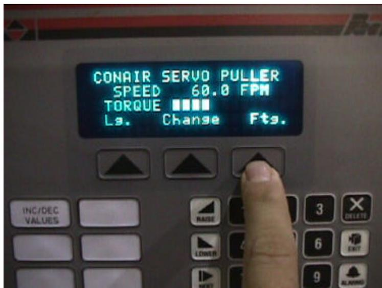
From the main screen with either Sm or Lg, push the button below the word **Ftg.** to access the Footage Counter screen.
